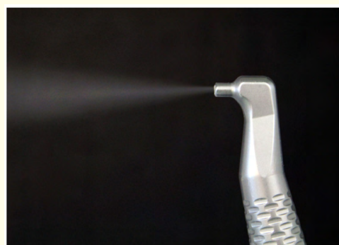
Figure 2: Blasting nozzle of PJD device.
