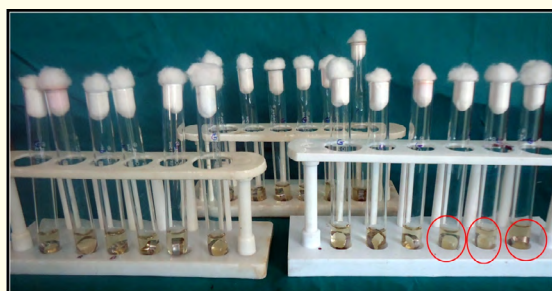
Figure 3: Group 2 (Glass bead sterilization) [Note: Highlighted test tubes shows presence of turbidity].
