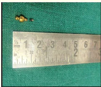
Figure 3: Retrieved screw of ball abutment.
