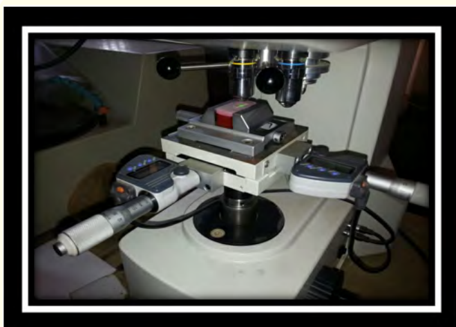
Figure 3: Specimen mounted on Vickers.
