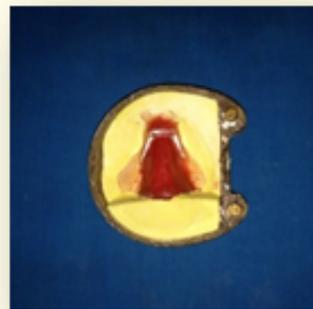
**Figure 5:** Sectional counter-flasking of the pattern.
