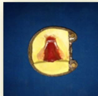
Figure 5: Sectional counter-flasking of the pattern.
