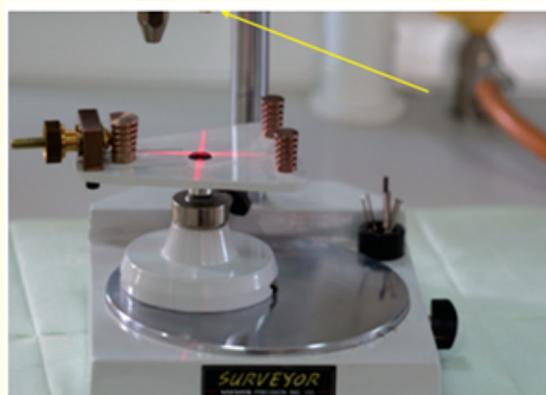
**Figure 8A:** Laser module fixed to dental surveyor.
