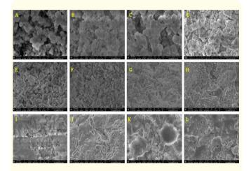
**Figure 1:** Scanning electron microscopy analysis of Bioedentine (A-D), EndoSequence (E-H), and Tech Biosealer(I-L) after exposure to PBS at a pH of 7.4 or butyric acid at a pH of 6,4, 5.4, and 4.4, respectively.
