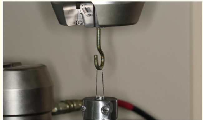
Figure 1: A specimen set-up in the Instron testing machine for a shear-peel bond strength test.
