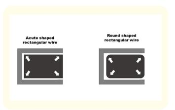
Using a test machine and a torque wrench they concluded that this variation is very important for the torque expression, since the play between the arch and the slot could cause a variation of 0.2 to 12.9 degrees in the same thickness. Analyzing the composition of the alloy, they concluded that the beta-titanium archs translated this difference more sharply than those of stainless steel and nickel-cobalt.
