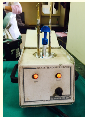
Figure 2: Glass Bead Sterilizer with common salt in which composite instruments are placed along with composite syringe.
