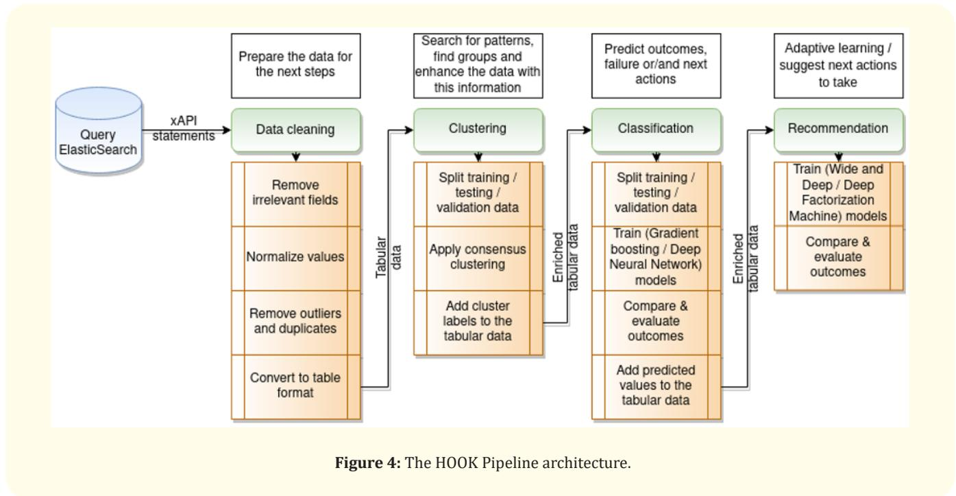
Figure 4: The HOOK Pipeline architecture.
