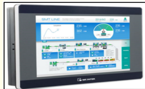
Figure 4: Example of HMI.
