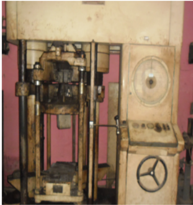
Figure 7: Pull-out test equipment.
