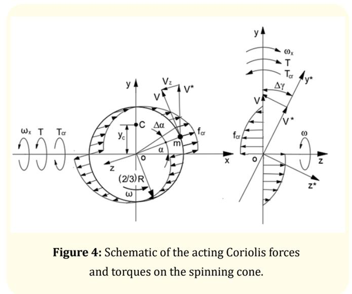
**Figure 4:** Schematic of the acting Coriolis forces and torques on the spinning cone.
