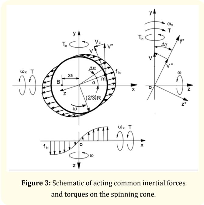
**Figure 3:** Schematic of acting common inertial forces and torques on the spinning cone.
