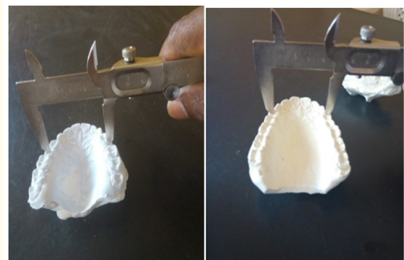
Figure 2: Picture of the measurement of first inter-premolar width and second inter-premolar width of the maxillary teeth.
