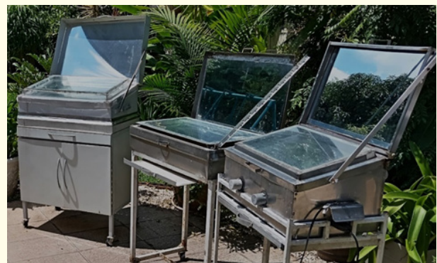
Photo 1: Some Solar Cookers/Ovens designed/studied and used by author at home.
