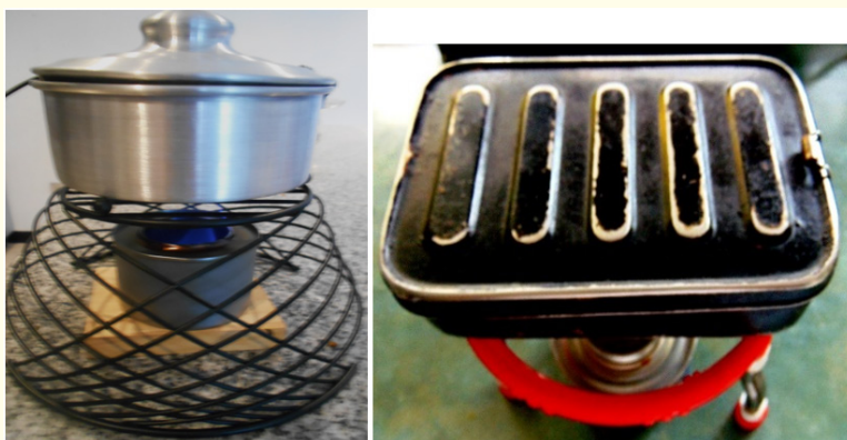
Photo 6: Heating of Pinto with Ethylene Glycol in Aluminum (left) and Steel (right) pot.
