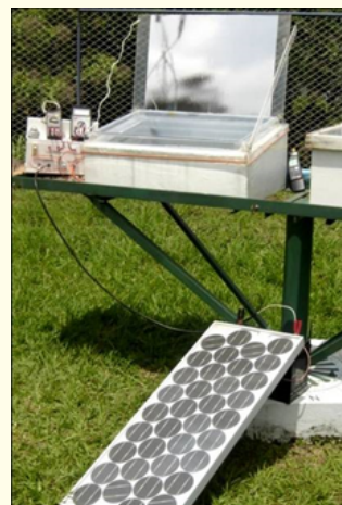
Photo 8: Solar Electric Oven with 12V PV panel.
