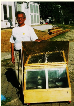
Photo 11: Two compartment Solar Oven, constructed and studied at Freiburg, Germany.
