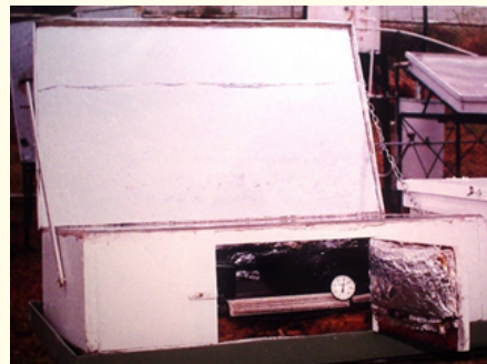
Photo 5: Sensible heat storage solar oven, using bricks.
