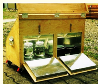
Photo 6: Latent heat storage solar oven, using Phase Change Material.
