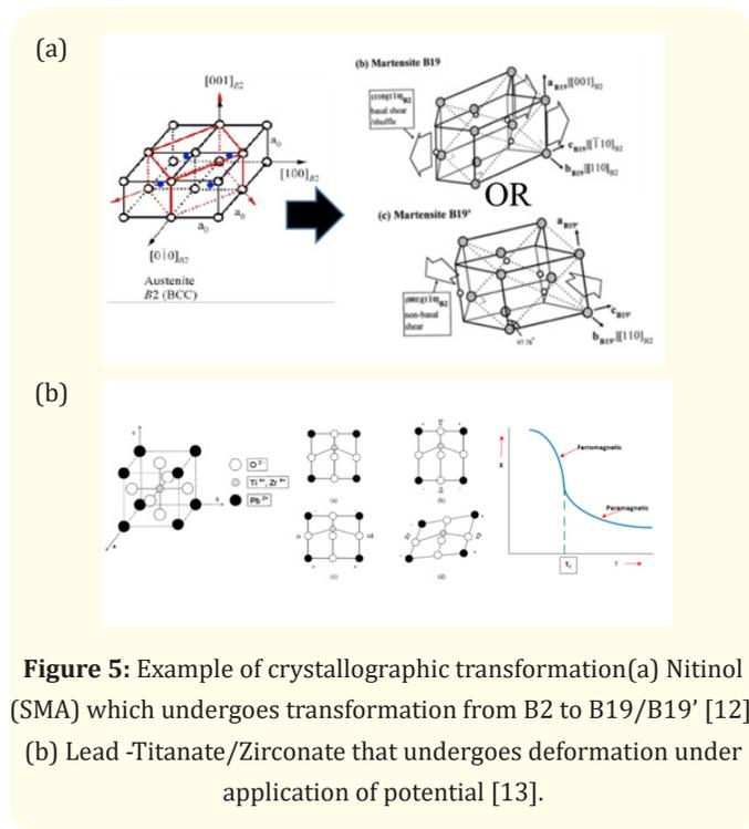
**Figure 5:** Example of crystallographic transformation(a) Nitinol (SMA) which undergoes transformation from B2 to B19/B19' [12], (b) Lead -Titanate/Zirconate that undergoes deformation under application of potential [13].
