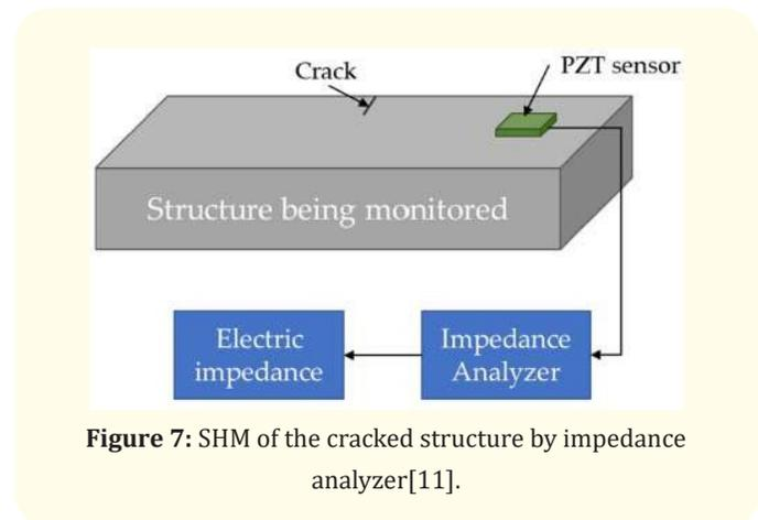
**Figure 7:** SHM of the cracked structure by impedance analyzer[11].
