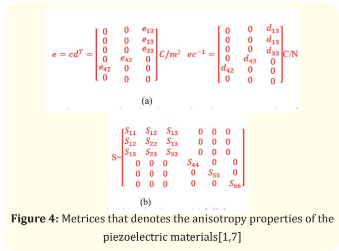
Figure 4: Matrices that denote the anisotropy properties of the piezoelectric materials[1,7]
