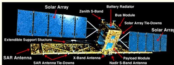
**Figure 4:** The photograph of Radarsat-1 satellite describing the placement of C-Band Synthetic Aperture Radar (SAR) [10].
