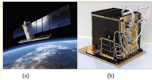
**Figure 14:** The photographs of (a) Sentinel-1 satellite and (b) electronic system of C-band Synthetic Aperture Radar (SAR) [5].
