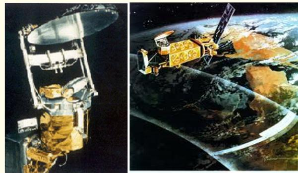
**Figure 19:** Image of Defence Meteorological Satellite Program (DMSP) satellite carrying Special Sensor Microwave Imager (SSM/I) [5].
