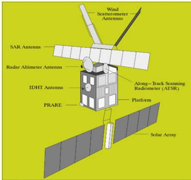
**Figure 12:** The photograph of European Remote Sensing Satellite-1 (ERS-1) satellite depicting onboard the placement of different Microwave Instruments [5].
