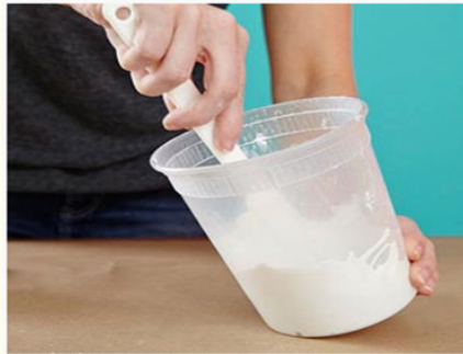
Figure 2: Pasty mixture (gypsum + water).
