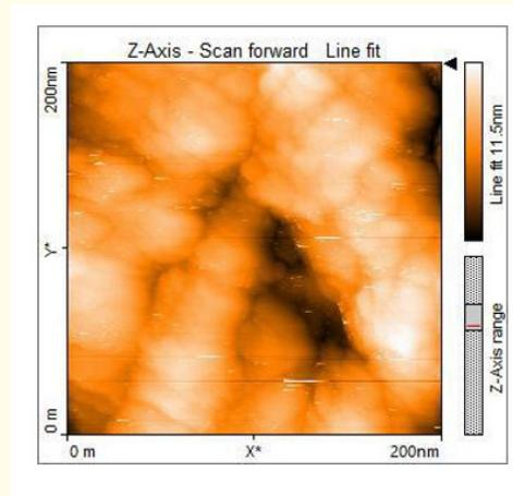
**Figure 4:** Measured STM topographic image of gold thin film using a mechanically cut STM tip.
