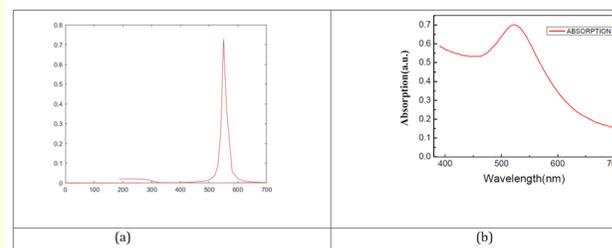
**Figure 2:** (a) Theoretical formulation showing absorption peak of Gold QDs, (b) UV-vis spectroscopy analysis of DDAB coated gold quantum dots dispersed in DI water.
