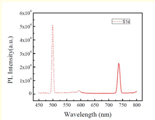
**Figure 3:** Photoluminescence analysis of DDAB coated gold quantum dots dispersed in deionized water the dotted graph shows excitation and the solid graph shows the emission spectra.
