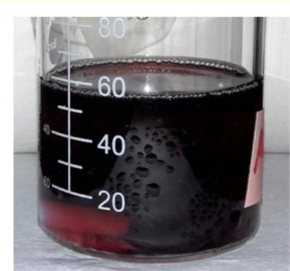
**Figure 1:** Photograph of as synthesized DDAB coated Au QDs solution.
