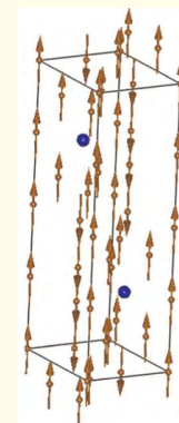
Figure 6: Magnetic structure of \text{BaFe}_{12-x}\text{Al}_x\text{O}_{19} on the basis of Gorter model: \text{Fe}^{3+} ion has magnetic moment, \text{Ba}^{2+} ion has no magnetic moment [39].
