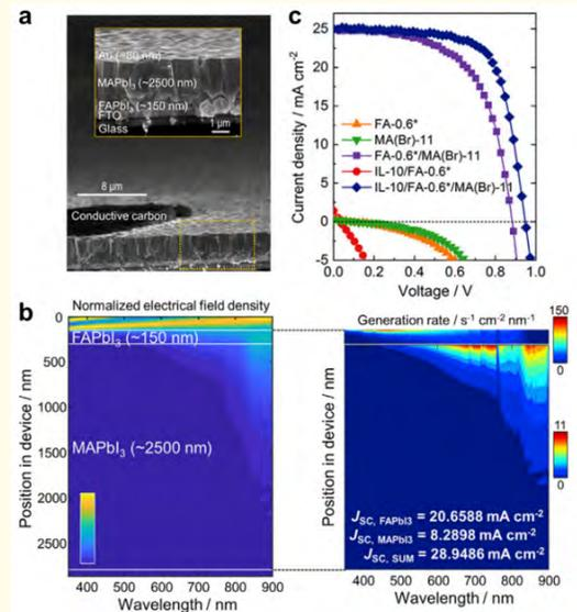
**Figure 1:** (a) Cross-sectional SEM images of the optimized CTL-free PSC. Inset shows the zoomed image. (b) Normalized electric field intensity distribution (left) and corresponding exciton generation rate distribution (right), determined from the transfer matrix model. (c) J-V curves of the PSCs based on different configurations. Adopted with permission from [6].
