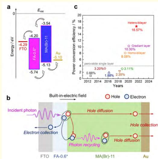
**Figure 2:** (a) Energy level alignment of the CTL-free PSC, derived from UPS results. (b) Working mechanism of CTL-free PSC. (c) Efficiency chart of CTL-free PSC. Adopted with permission from [6].
