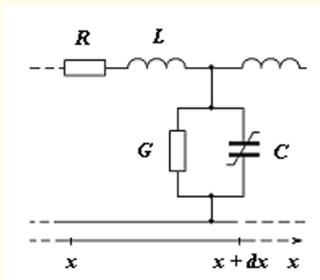
Figure 1: Element of long line with magnetic coupling.
