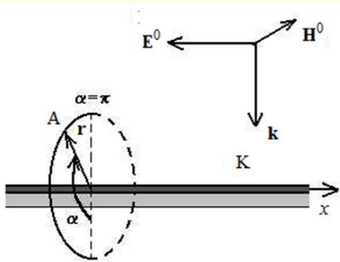
**Figure 1:** Scheme of the statement of the problem of diffraction on a cylindrical object: A is a point, in which the field is calculated; K is a cylindrical object.
