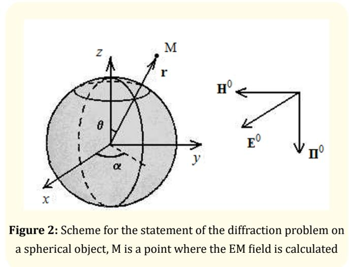
**Figure 2:** Scheme for the statement of the diffraction problem on a spherical object, M is a point where the EM field is calculated
