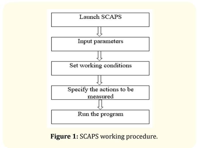
Figure 1: SCAPS working procedure.
