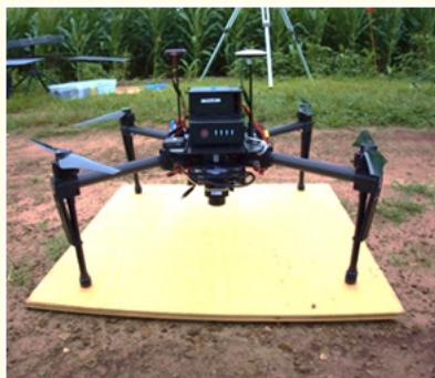
Figure 1: Matrice 100 quadcopter was used for infrared data collection.
