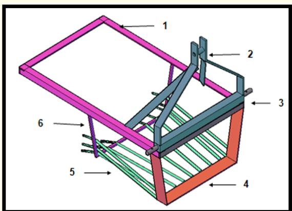
**Figure 1:** Complete isometric view of tuber crop harvester.
