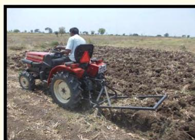
**Figure 2:** Small size tractor operated tuber crop harvester in operation.
