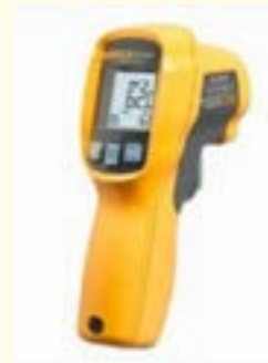
Figure 1: Canopy temperature for some crop using infrared thermometer.
