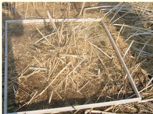
Figure 1: A quadrat, a meter square of wood, is being thrown randomly to take samples of the residues for each tillage method.
