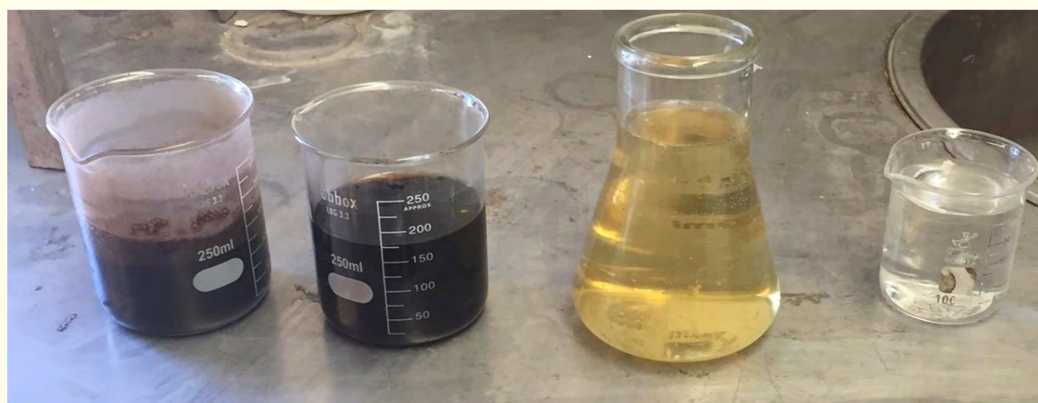
Figure 1: From left to right: Initial Wastewater, filtered by Ultrafiltration, by Nanofiltration and by Reverse Osmosis.
