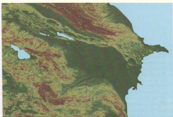
Figure 2: Angular slopes map developed in accordance with method S lope based on a digital model of Azerbaijan hypsometric.
