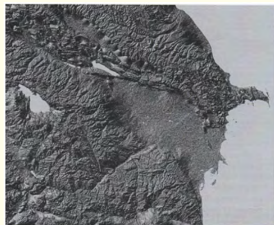
Figure 4: Image obtained due to overlapping shadow effect on a digital surface model territory.
