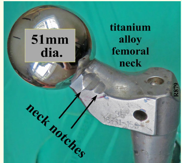
Figure 3: Twin notches on retrieved THA femoral-neck (titanium-alloy), 51 mm SRM case presented by permission of J. Recon. Review [Donaldson, 2015].
