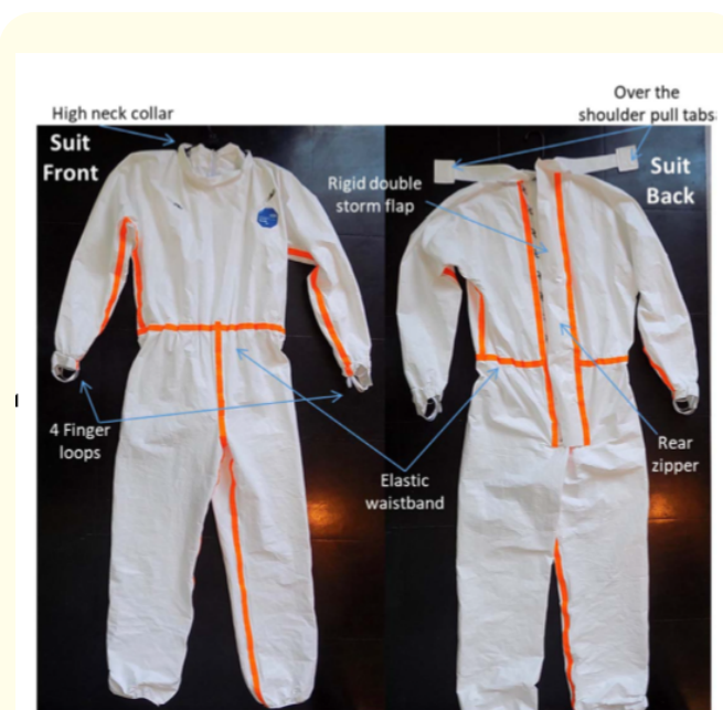
Figure 2: Center for Bioengineering Innovation and Design/Jhpiego personal protective equipment ensemble.
