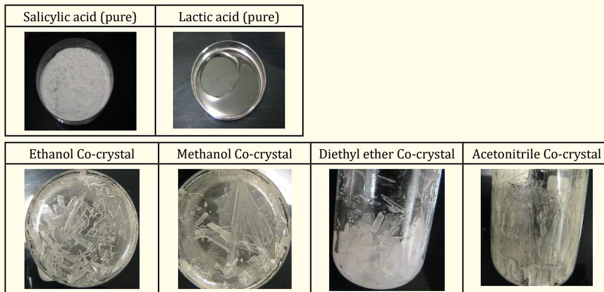
**Figure 3:** Co-crystals obtained from each co-solvent/Reflux technique.
