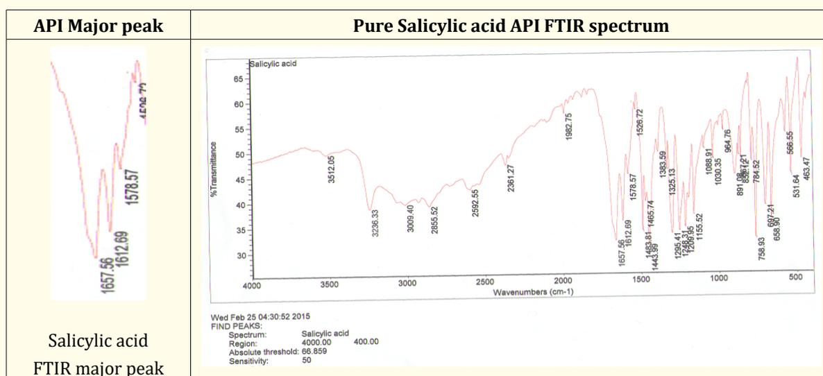
Figure 4: Pure Salicylic acid FTIR spectrum.
