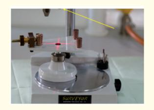
Figure 8A: Laser module fixed to dental surveyor.
