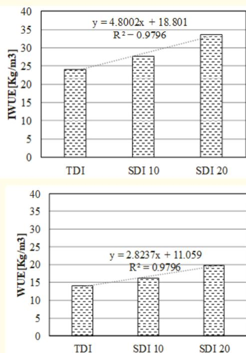
**Figure 6:** Effect of drip lateral depth on water use efficiency (WUE) and irrigation water use efficiency (IWUE).
