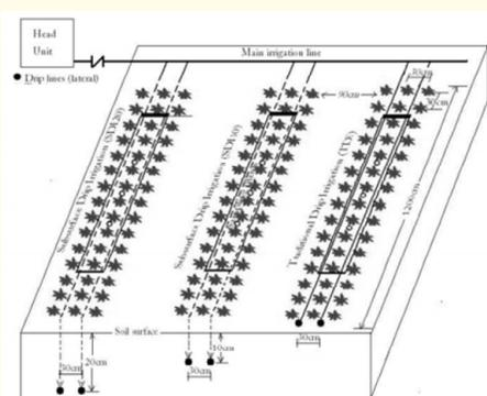
**Figure 1:** Eggplant spacing and drip line placement in the experiment.
